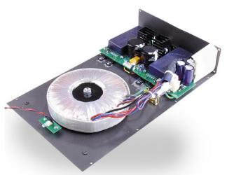
Hum may also be an issue with the GCHA if placed too close to a sensitive piece of equipment such as a phono preamplifier or turntable. The GCHA has an exceptionally large power transformer inside. This transformer can generate a fairly large magnetic field which can induce hum into sensitive equipment in close proximity.
