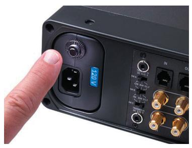
service representative. Should the Power Plant Premier cease to function, check the circuit breaker and if that fails, contact your dealer or PS Audio's service center for help.
